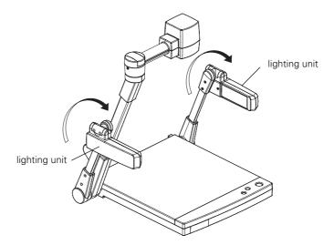
5. Tilt the lighting arms outward until they stop; then position the lighting units so that they face the stage (downward).
